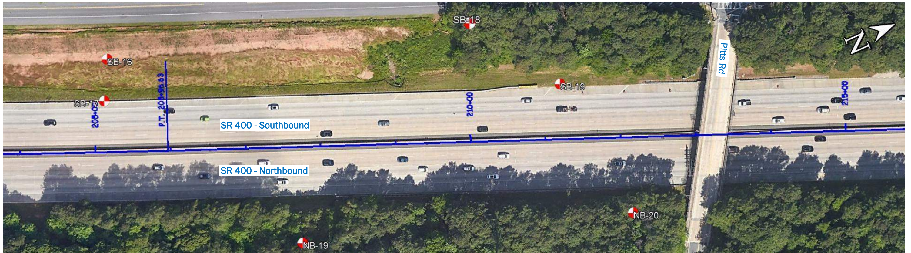
FIGURE 3-5 STATION 195+00 TO 215+00 BORING LOCATION PLAN SOURCE: Google Earth Aerial Photos SCALE: Not to Scale
